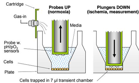
Figure 1. Adaptation of XF24 for in-vitro simulated IR model.
