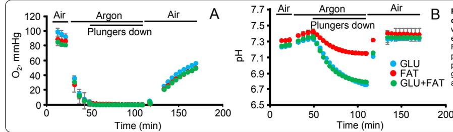
Figure 3. Typical XF24 pO<sub>2</sub> and pH traces during simulated IR. pO<sub>2</sub> (A) and pH (B) were measured by fluorescent probes embedded in the plunger in each well. Plungers were lowered for 60 min. in the presence of argon flow to simulate ischemia. pO<sub>2</sub> and pH from all wells within the same groups were averaged and data are shown as means ± S.D., for a single plate.
